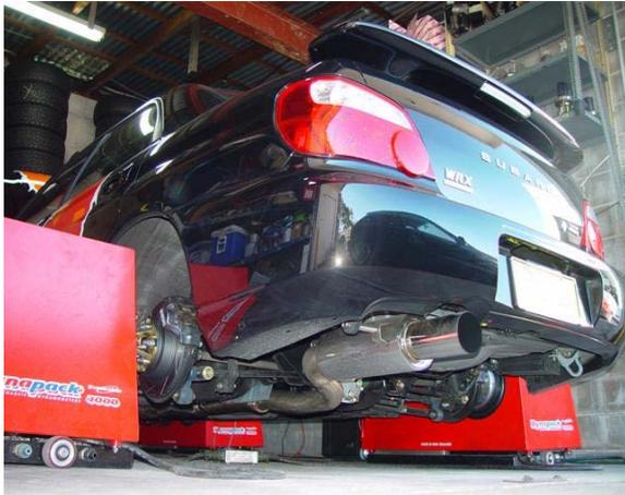
Into the bin goes the standard engine pipe and centre pipe – in its place are a new custom designed dump pipe from the turbo back, complete with custom designed splitter for improved response and high flow cat converter. A new 3” centre pipe completes the system, mounting up nicely to the upgraded 3” muffler fitted initially as part of the XA Kit.
