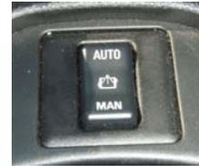
This switch in the centre console must be set to AUTO (blue light on RHS of dash will illuminate when system is active).
